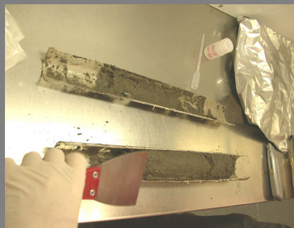
Figure 2: Sampling the core.
