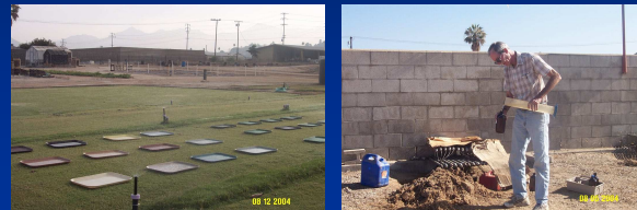
Figure 1. Retrofitted turfgrass plots and leachate collection for NDMA analysis
